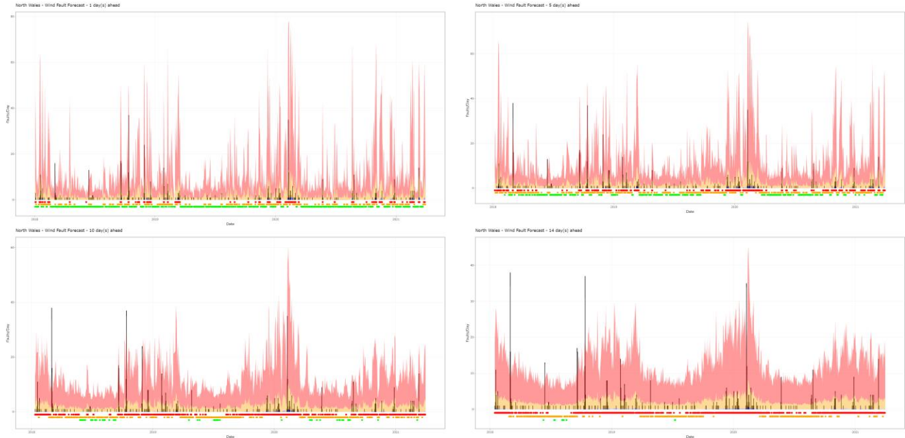
Figure 10: Fault forecasts for North Wales for 2018 to mid-2021. Day-ahead (top-left), five-days-ahead (top-right), ten-days-ahead (bottom-left) and 14—days-ahead (bottom-right) are illustrated for the whole period. The key is the same as that for Figure 4. Day-ahead forecasts are the most specific in terms of timing of large fault events (red spikes) and confidently predicting no faults (green). By 14-days-ahead, the forecast contains little specific information beyond average conditions for the time of year.
